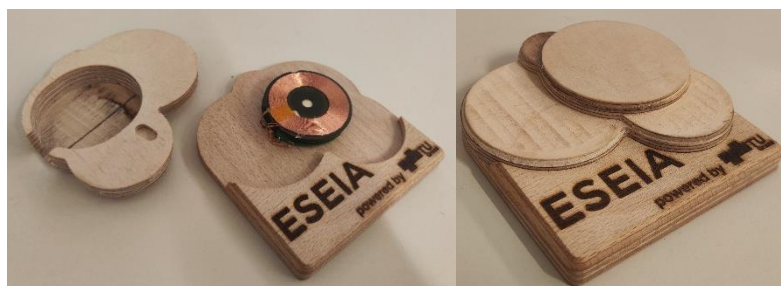
Fig 2: Raw base plate, charging module, logo in the making
